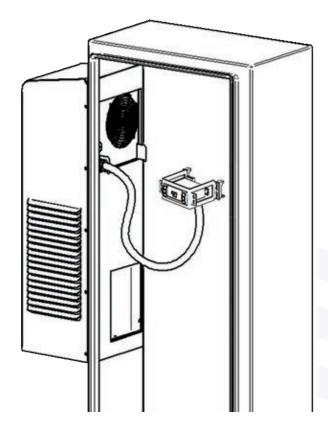
The side tabs located on each side of the controller face plate will be used for mounting to the server rack. Two din rail clips with four screws will be provided for din rail mounting applications.
