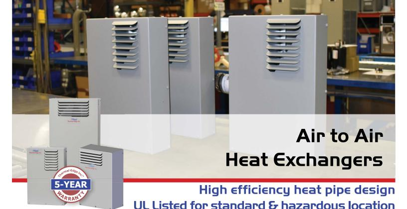
Thermal Edge Air to Air Heat Exchangers are a closed loop cooling system which employs the heat pipe principle to exchange heat from an electrical enclosure to the outside. Where ambient temperatures are suitable for heat pipes, they are the most efficient method of cooling as the waste heat is the engine which drives the system. The only power requirement is to operate two circulating fans or blowers.
