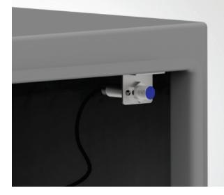
The Thermal Edge Open Door Kill Switch is designed to automatically shut off the enclosure air conditioner when the door of the enclosure is opened. When the door is closed, the air conditioner will resume normal operation. Each door switch is supplied with a 7-foot low-voltage cable and a mounting bracket.
