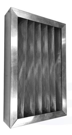
Thermal Edge offers extended surface, 2" deep replacement filters. These 250 micron stainless steel mesh filters, with 94% efficiency, extend the filter capacity by 400%. The filters are washable and reusable. Life expectancy is determined by the environment and the cleaning procedures. Stainless steel filters are preferred in wash-down applications over aluminum filters.
