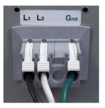
4 – If wires need to be removed, raise the lever directly above each wire to release it.
