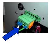
6 - If wires need to be removed from the male connector, insert a small screwdriver or pick into the hole directly above each wire and push to release it.
