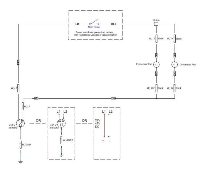
Note: Schematic applies to all voltages; DC voltages do not have ground wire.
