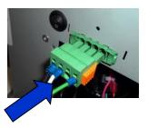
6 – If wires need to be removed from the male connector, insert a small screwdriver or pick into the hole directly above each wire and push to release it.
