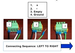
**NOTE:** If using stranded wires, it may be difficult to insert into the receptacles without releasing the spring tension as described below in the removal instructions. The wires can be tinned or pin terminals (as shown above) or pin ferrules may be attached to stranded wires to ease insertion into the receptacles.
