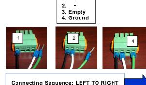
**NOTE:** If using stranded wires, it may be difficult to insert into the receptacles without releasing the spring tension as described below in the removal instructions. The wires can be tinned or pin terminals (as shown above) or pin ferrules may be attached to stranded wires to ease insertion into the receptacles.
