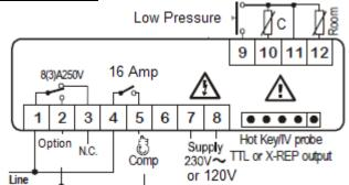
*Note:* Schematics applies to all voltages; optional accessories wiring not provided in this document. If you require electrical schematic with options contact our technical support and provide your model number.
