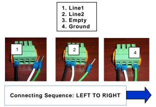
**NOTE:** If using stranded wires, it may be difficult to insert into the receptacles without releasing the spring tension as described below in the removal instructions. The wires can be tinned or pin terminals (as shown above) or pin ferrules may be attached to stranded wires to ease insertion into the receptacles.
