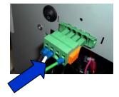
6 – If wires need to be removed from the male connector, insert a small screwdriver or pick into the hole directly above each wire and push to release it.
