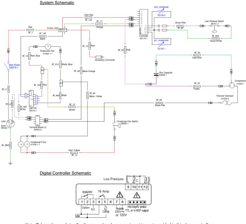
*Note:* Schematics apply to all voltages; optional accessories wiring not provided in this document. If you require electrical schematic with options contact our technical support and provide your model number.
