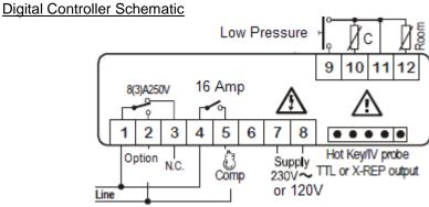
*Note:* Schematics applies to all voltages; optional accessories wiring not provided in this document. If you require electrical schematic with options contact our technical support and provide your model number.
